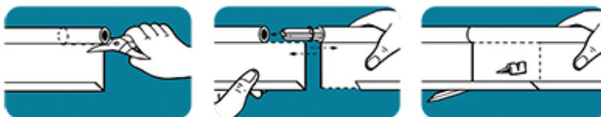
1. Cut off a 4" section of the round bead on one of the edging pieces and a 4" section of the v-lip on the other piece with a metal snip, utility knife or saw.
